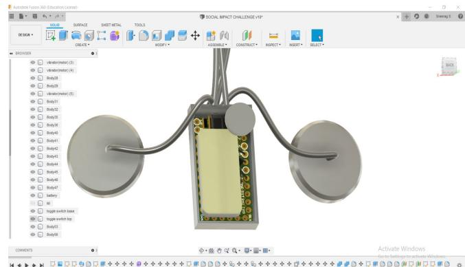
These vibrators are made to vibrate sequentially by connecting them to an Arduino pro mini ATMEGA328P 5V/16M. Using the Arduino mini, we can program the board to make the top two vibrators vibrate first and as they stop the 2 vibrators below it start vibrating. Now as they stop the other ones below it starts vibrating. Now the cycle again repeats. Thus this gives a massaging to the user for about 15seconds to 20seconds time.
